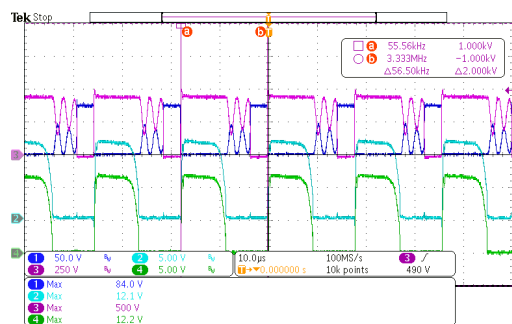
Fig.140 230Vac/50Hz; 20V; 100% Load, Ch1: SR MOS Drain. Ch2: SR MOS Gate. Ch3: U1 Vds. Ch4: SR IC VG.
