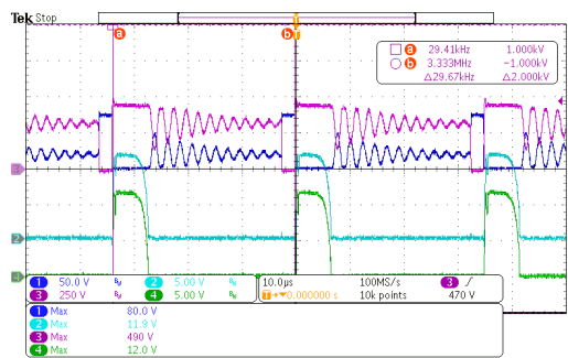
Fig.137 230Vac/50Hz; 20V; 25% Load, Ch1: SR MOS Drain. Ch2: SR MOS Gate. Ch3: U1 Vds. Ch4: SR IC VG.
